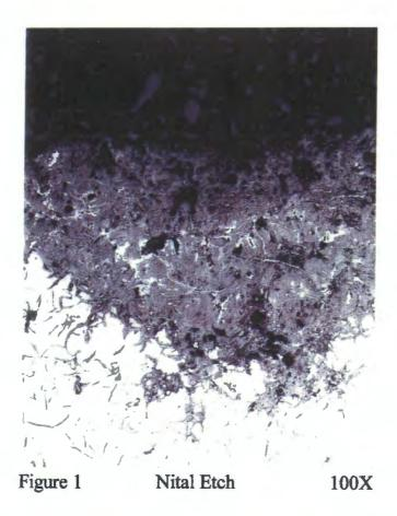
Photomicrograph of graphitic corrosion on the specimen from Site 7.
